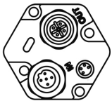
5 pin M12 connector (2x) + 4 pin M8 connector
