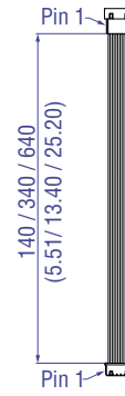
Extension cable molex to molex 140 mm: Part no. 254 642-1 340 mm: Part no. 254 642-2 640 mm: Part no. 254 642-3
