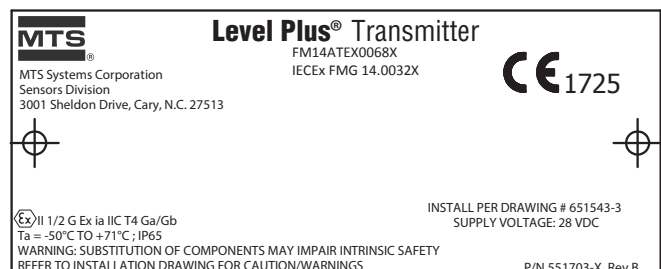
Fig. 31: ATEX/IECEx label, Modbus and DDA
