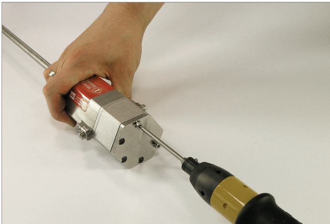
1 Loosen the five M4×10 screws (A/F 3).
