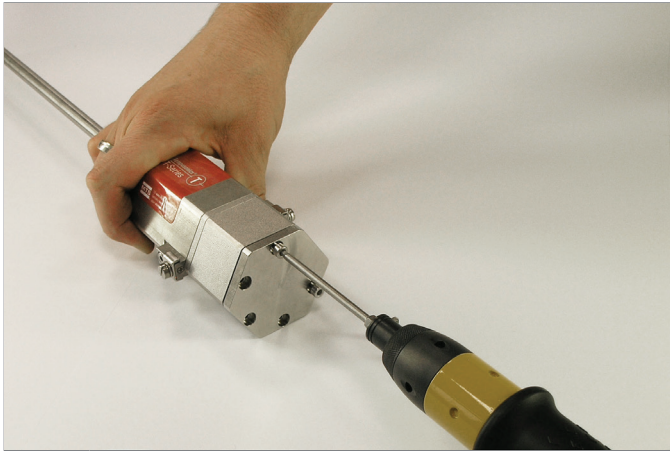
1 Loosen the five M4×10 screws (A/F 3). Remove the upper lid. Loosen the six M4×40 screws (A/F 3) of the connection adapter. Remove the connection adapter. See also Fig. 6.
