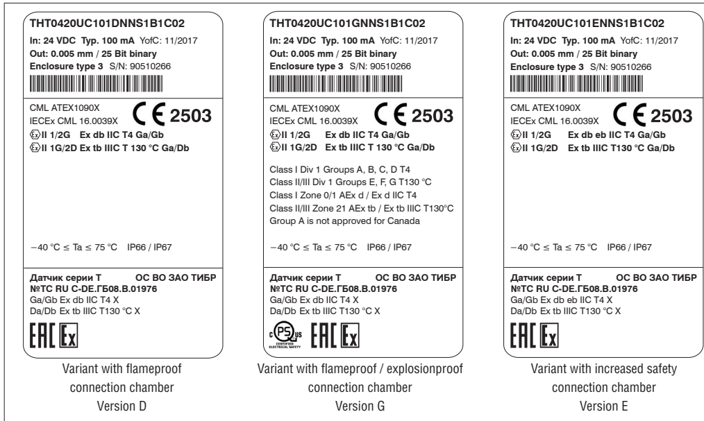
Fig. 1: Example of a nameplate of a TH sensor
