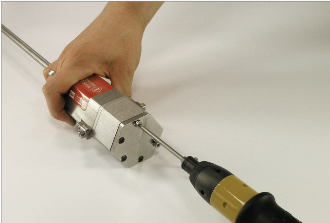
1 Loosen the five M4×10 screws (A/F 3).
