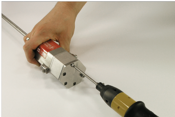
1 Loosen the five M4×10 screws (SW 3).
