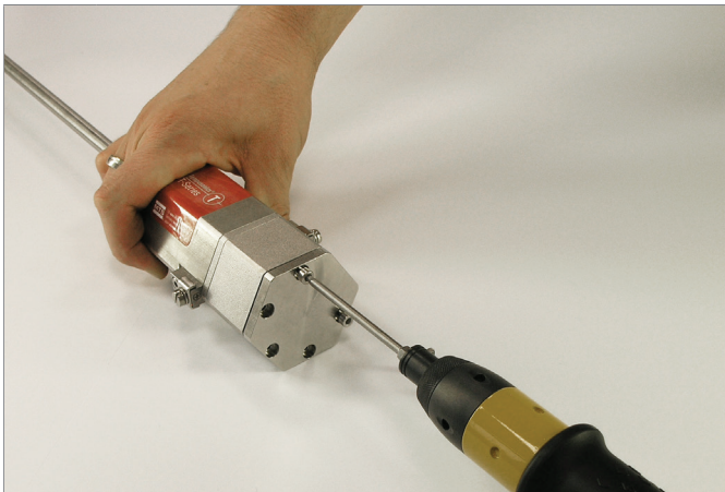
1 Loosen the five M4×10 screws (AF 3).
